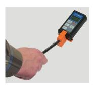
The radiation monitors are microprocessor instruments with digital readout. The G-M tube with the energy compensating filter is used is a detector.
