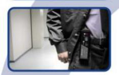
The instruments detect standard samples of nuclear materials at a distance of  $(100 \pm 5) \cdot 10^{-2}$  m from detector's sensitive surface (detection threshold for Pu - 3.0 g, U - 250 a) that corresponds to the minimum detectable radionuclide activity radioactive nuclide: <sup>137</sup>Cs 0.6 MBa, <sup>133</sup>Ba 0.33 MBa, <sup>60</sup>Co 0.3 MBq.
