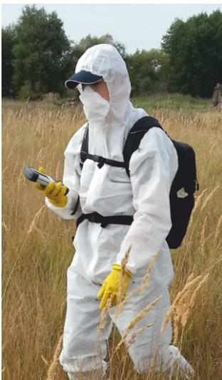
As a control and indication device the handheld computer (HPC) is used. Data transfer from detection units to HPC is carried out via Bluetooth. Data transfer by cable is carried out in the places where transfer via radiochannel is impossible or undesirable.
