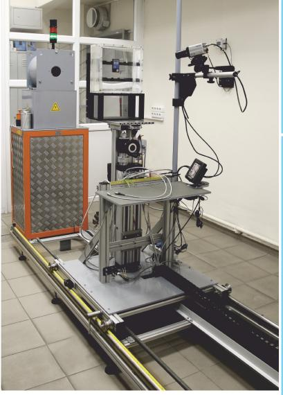
Reference gamma beam irradiator with calibration bench is designed to simulate and transmit air kerma, exposure dose, individual dose equivalent and dose equivalent units and their respective rates into working standards and measurement instruments during verification, calibration and test procedures.
